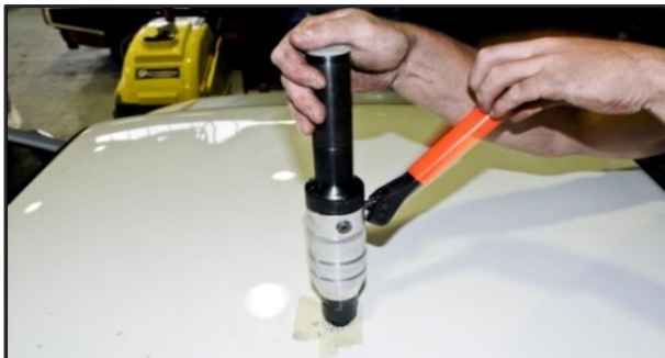
12mm hole drilled through the roof.
