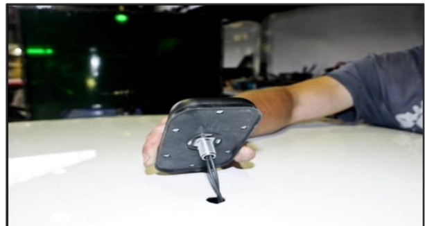
Antenna leads passed through the hole.
