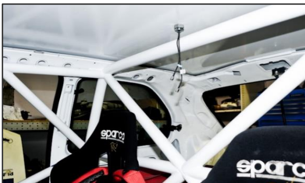
Nut used to secure antenna to roof.
