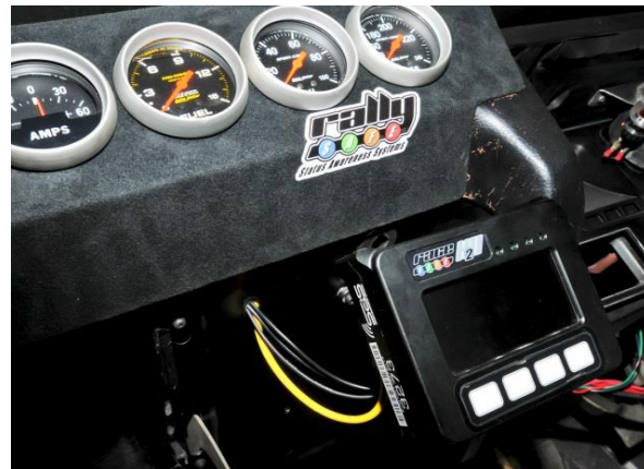
The RallySafe unit then mounts to the 25mm rubber ball mount using the adjustable mount connector.
