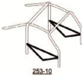
Drawing of the doors reinforcement
