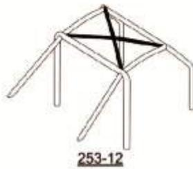
Drawing of the roof reinforcement
