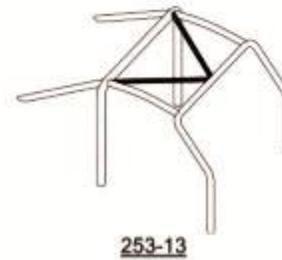
Drawing of the roof reinforcement
