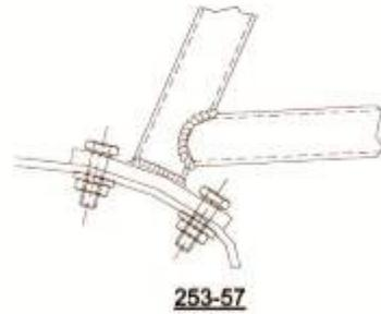
Drawing showing how to screw the fixing plate
