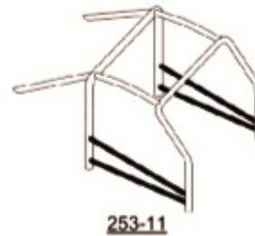
Drawing of the doors reinforcement
