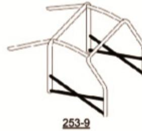
Drawing of the doors reinforcement
