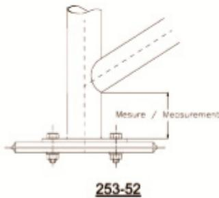
Drawing showing how to screw the fixing plate
